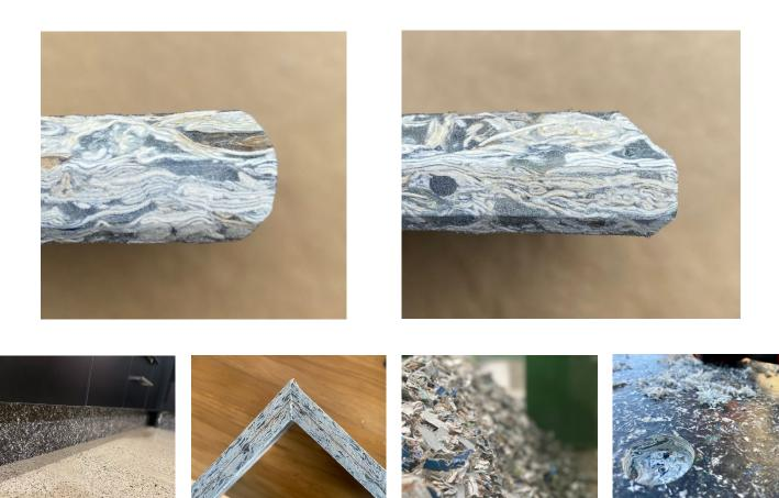
**Colouring** of the edge can be made by colouring the epoxy to achieve a matching or contrast colour to the facing. For small applications the use of food colouring is an option to colour the epoxy.
