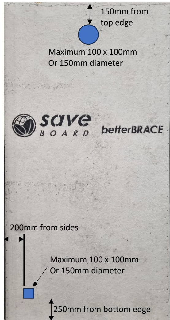
DIAGRAM 2 – Permitted penetrations in Bracing board. Note: All penetrations are to be sealed as per the instructions in this guide.
