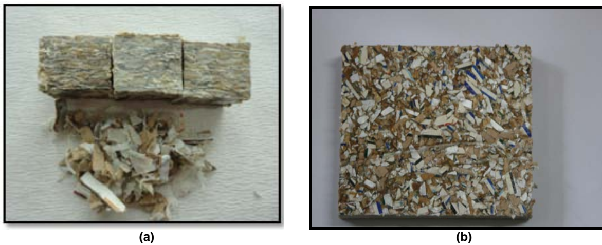
Figure 1. Shredded particles (a) and panel specimen manufactured (b)
